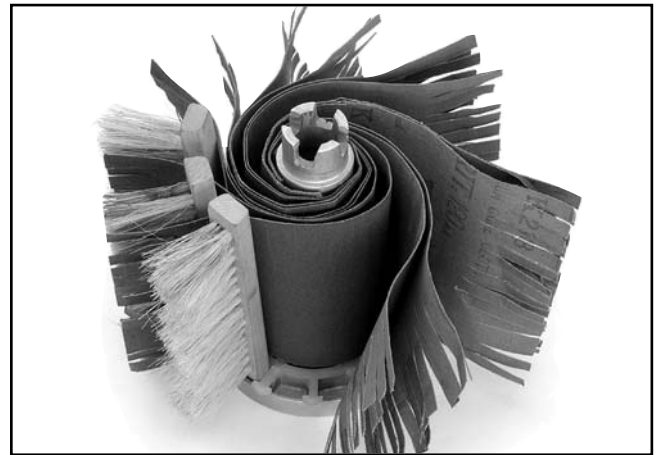
Figure 25. Re-assembling the flap sander.
